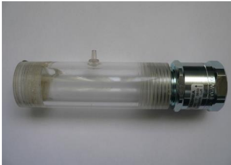
Figure 3. EFV mounted with a transparent plexiglass pipe for monitoring flow cut-off behavior
