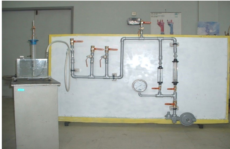
Figure 2. The EFV testing setup integrated with the leakage measurement unit
